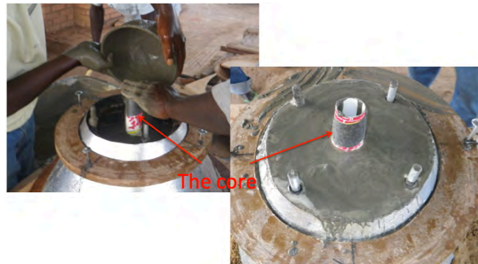
Figure 40: Metal cone around the cage, and secured with wires Figure 41: Pouring concrete
