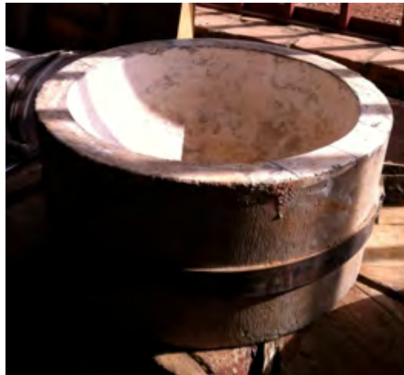
Figure 27: Male Mold Cavity
