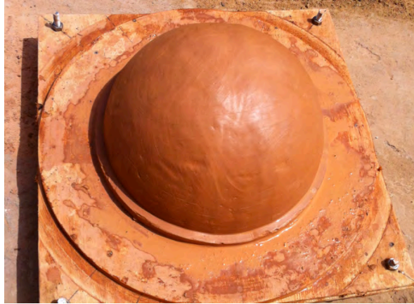
Figure 38: Finished prototype filter element
