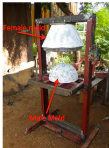
Figure 20: Pure Home Water's 1 st Mani Press showing FM and MM
