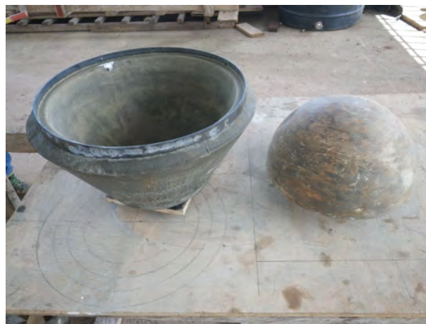
Figure 49: Finished female mold (left) and male mold (right)
