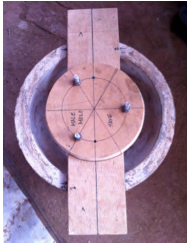
Figure 46: Wooden Template A at the center of Male Mold Cavity
