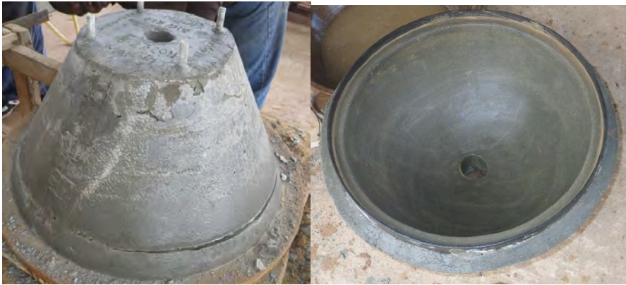
Figure 42: Finished Female Mold, except that the hole is unfilled
