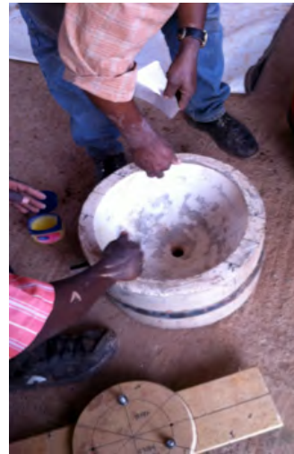
Figure 44: On the underside of Wooden Template A Figure 45: Apply Vaseline to Male Mold Cavity
